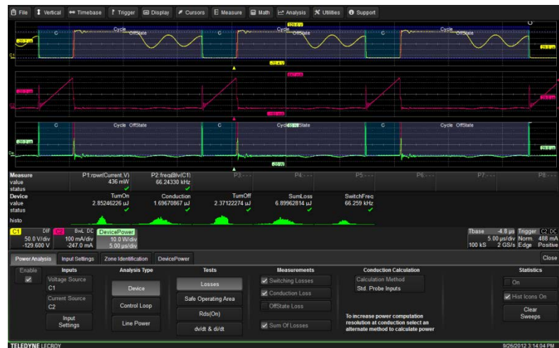
Figure 1: An example of the Power Analyzer option with a choice of Device, Control Loop, and Line Power Analysis
