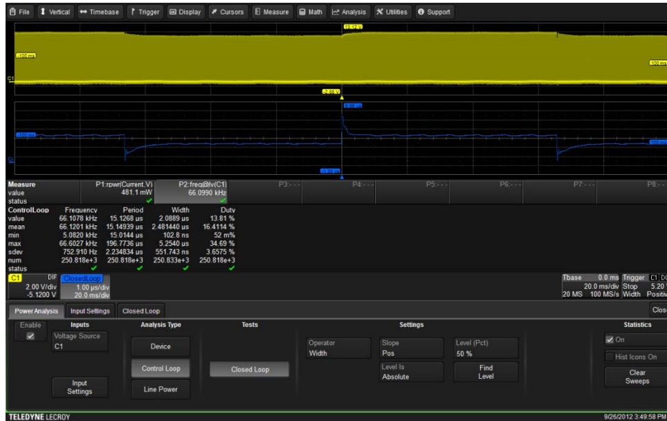
Figure 3: Closed loop analysis of the gate drive waveform for a switched mode power supply shows the variation in gate drive pulse width in response to a change in power supply loading
