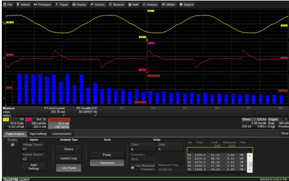
Figure 4: Line power analysis showing the harmonics of line current. The table in the lower right lists each of 40 harmonics including it's frequency and level
