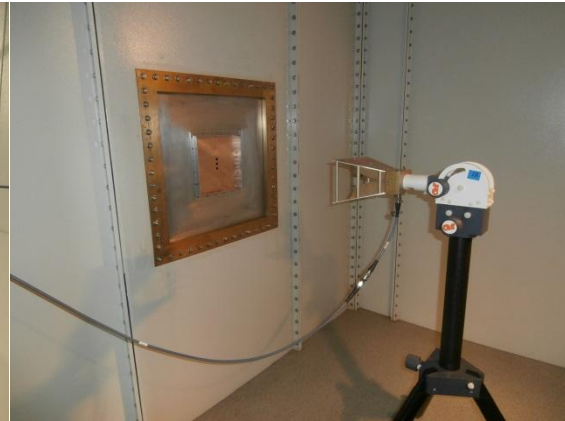
Figure 5 Test set-up in receiving room
