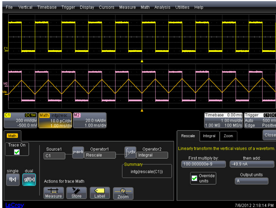
Figure 4: Using the rescale constant to remove the mean value of the waveform in Channel 1 before integrating
