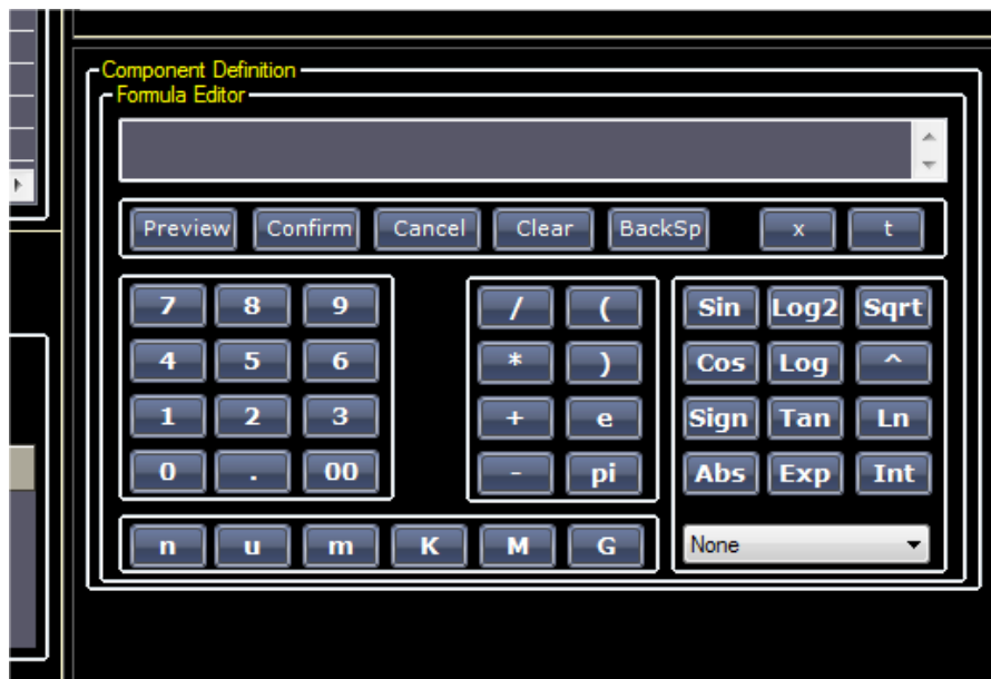
Figure 6: The formula editor allows you to build a waveform analytically using equations. Equation can be based on time (t) or samples (x)
