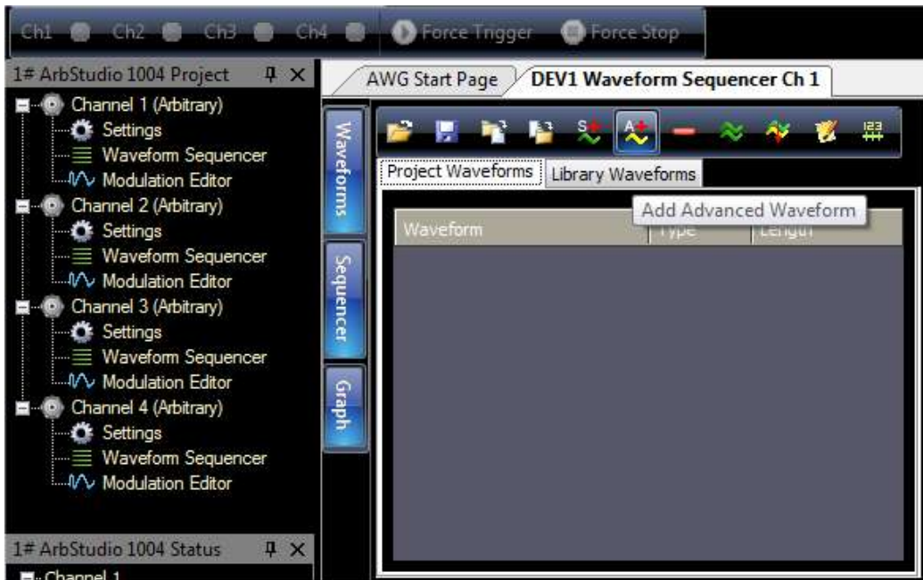
Figure 2: Double clicking on the Waveform Sequencer under one of the channel will open the Waveform sequencer window
