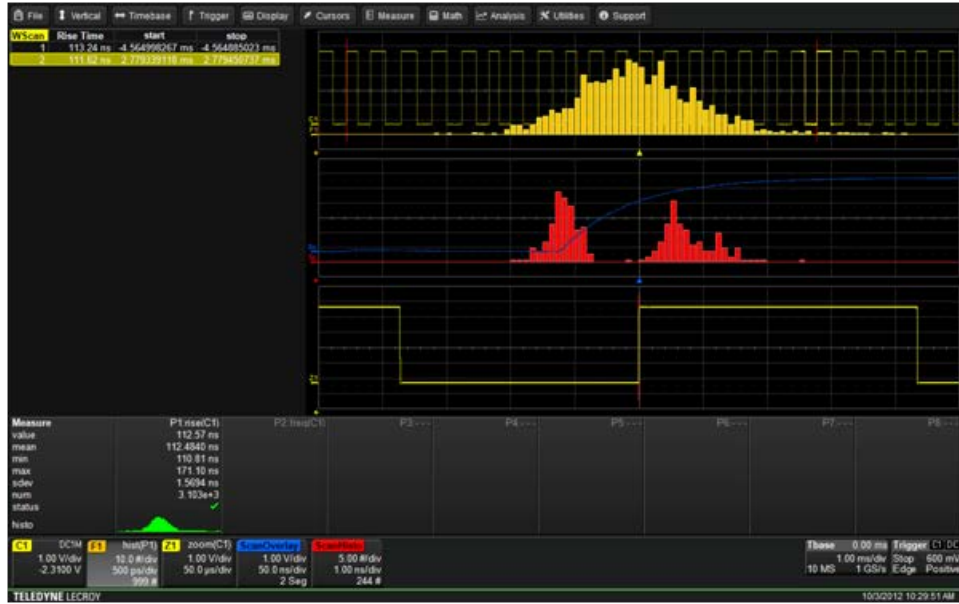
Figure 3: Shown is WaveScan in Measurement mode and filtering for the smallest and largest rise times in the signal trace
