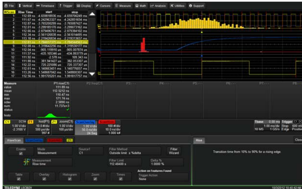
Figure 4: WaveScan’s Histogram function enables HDO6000 oscilloscopes to create a persistence display of only the results that meet the users’ predefined criteria. This is shown in the blue trace in the center grid
