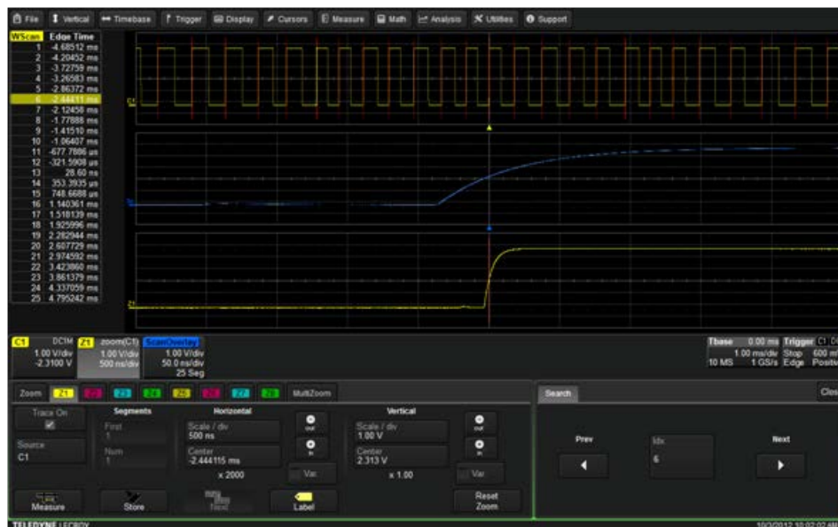
Figure 2: Tapping any line in the WaveScan table changes the zoom view to the corresponding event
