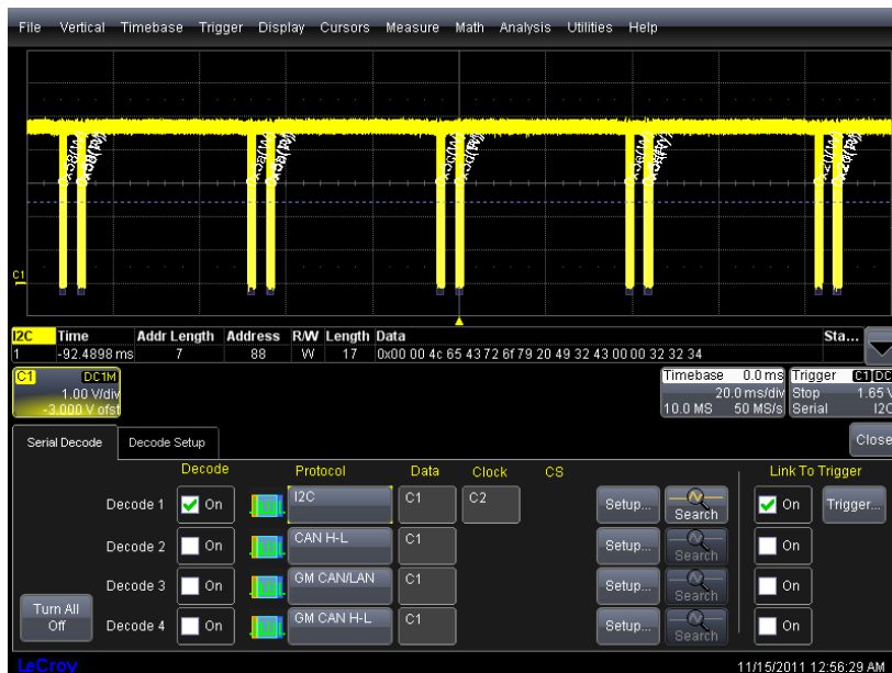
Figure 4: Setting up I2C decode using the serial decode dialog box
