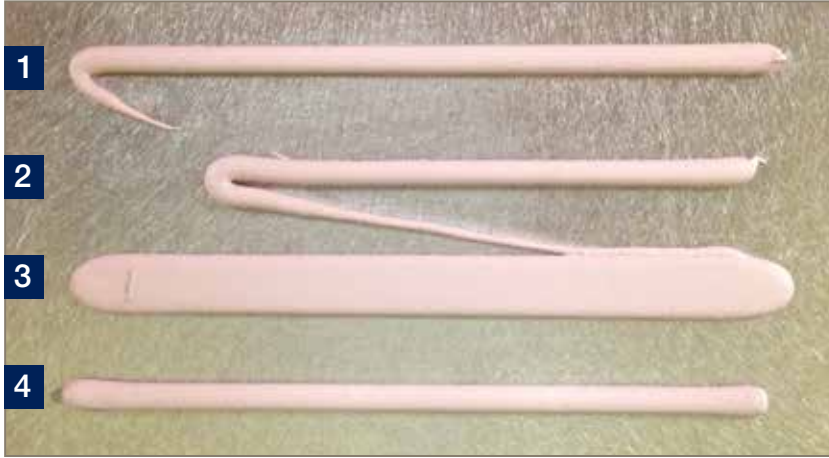
Figure 6: Common Line Dispensing Concerns Common dispensing issues: (1, top) system did not have a program for bead termination; (2, middle top) needle was too high and there was no bead termination programmed; (3, middle bottom) needle too low; (4, bottom) correct height with bead termination.
