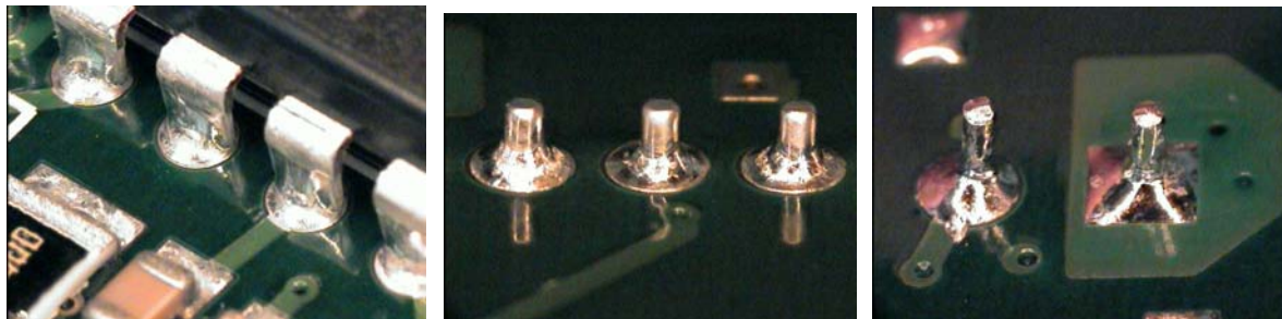
Figure 7. Various through-hole parts showing excellent wetting on top and bottom-side
