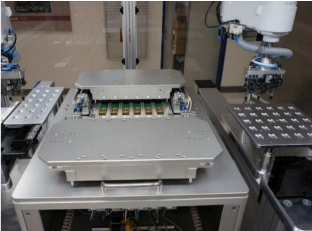
Figure 32: Automatic test equipment for module test
