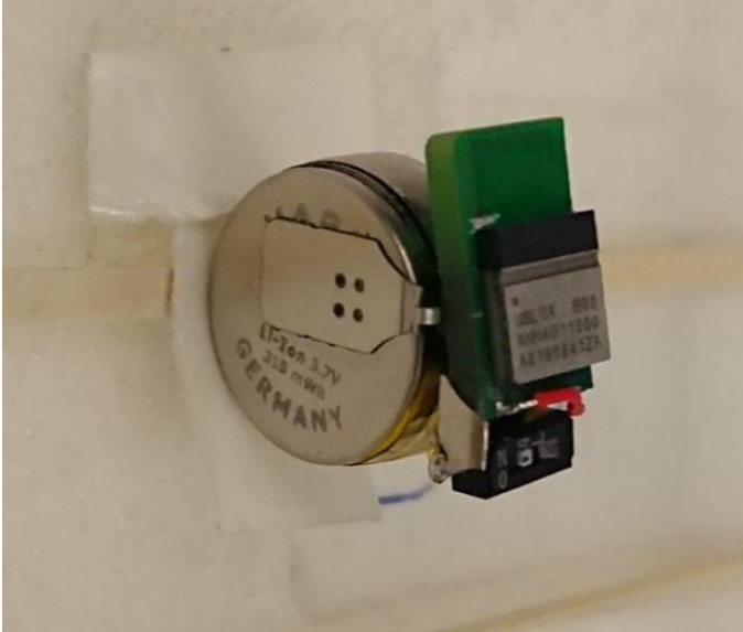
Figure 42: A tiny ANNA-B1 application including coin cell battery
