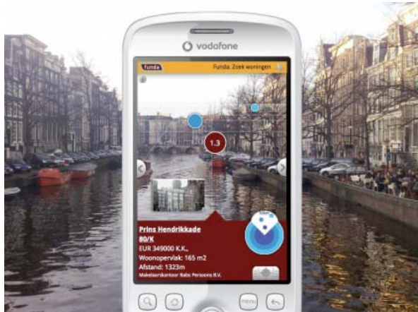
Figure 5. In this application of augmented reality by Layar, knowledge of one's position and heading are used to layer POI information on top of the information being received by the handset's camera. 9
