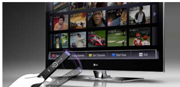
Figure 3. The LG Electronics Magic Motion™ remote uses motion processing for menu navigation and control of other functions. 6
