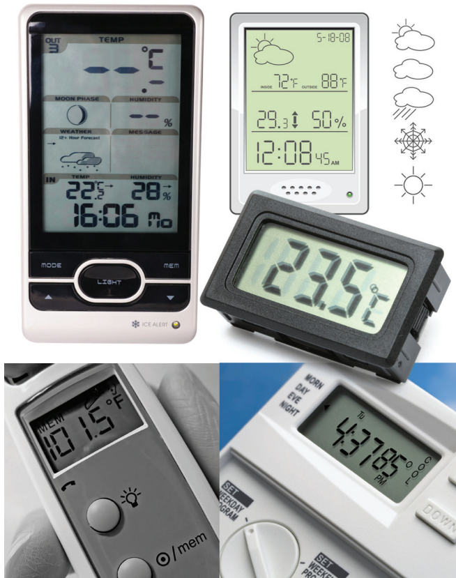
Figure 1. A microcontroller featuring an RC analog-to-digital converter is a cost-effective means of calculating temperature and humidity in portable instruments, weather stations and thermostats.
