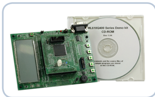
Figure 5. The Demo Kit provides an effective means of evaluating the features of the ML610400 family of devices.
