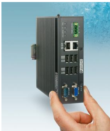
Figure 1: Example of a compact industrial box PC with CompactFlash (CF) mass storage.
