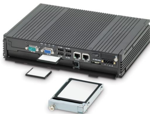
Figure 2: Easy accessible mass storage drives increase serviceability.
