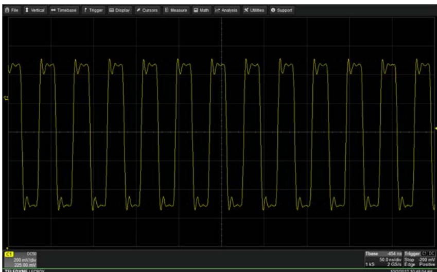
Figure 1: This is the initial setup with a 25-MHz clock waveform on Channel 1 of the HDO oscilloscope.
