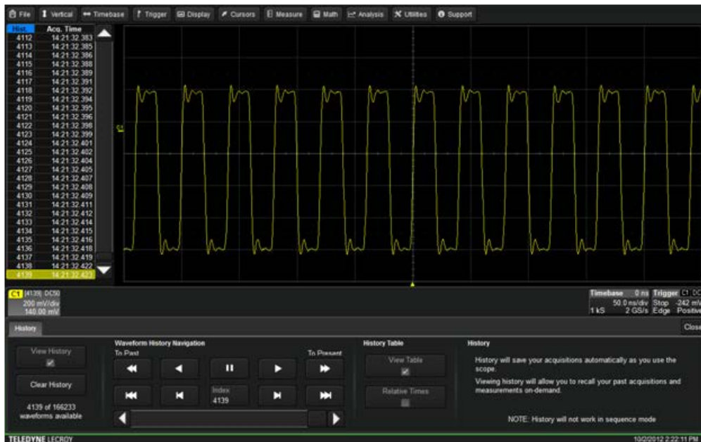
Figure 3: Checking both View History and View Table brings up the History Mode table seen at top left. History Mode saves and shows all acquisitions automatically with the time at which they were acquired.
