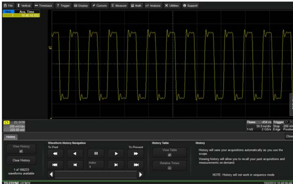
Figure 2: Upon invoking the History Mode option in the Timebase pulldown menu, users are presented with the controls dialog at the bottom of the screen.
