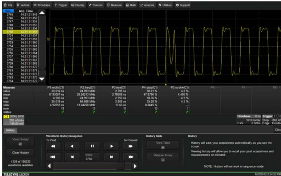
Figure 5: Measurement and/or math operations may be performed on any acquired waveform in History Mode. In this example, one of a group of single-shot acquisitions is measured for width, frequency, rise time (20-80%), duty cycle, and overshoot. Note that the measurement statistics show the 4.49-ns glitch
