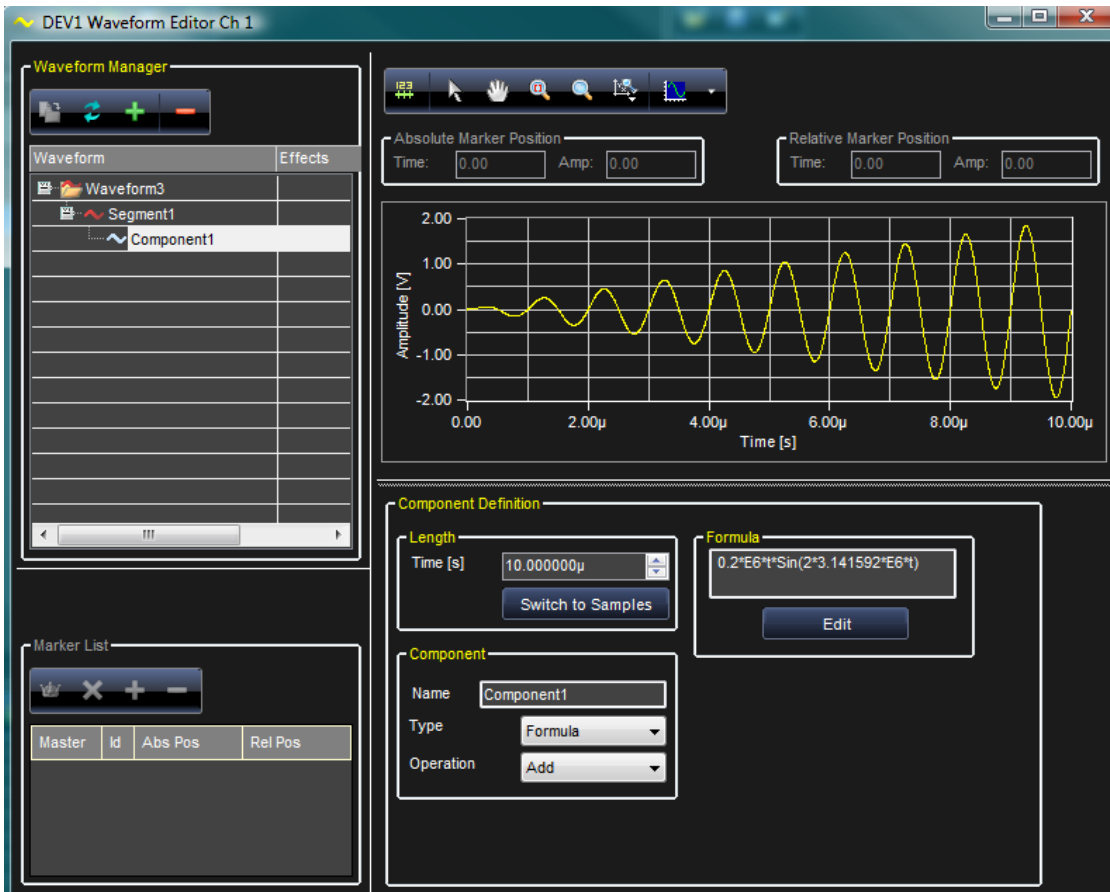
Figure 3-10. A linear amplitude sweep of a 1 MHz sine waveform. The actual formula used here is 0.2 \times 10^6 t \sin(2 \times 3.141592 \times 10^6 t) . Set the time to 10.000000 \mu s to view the graph as previously shown.
