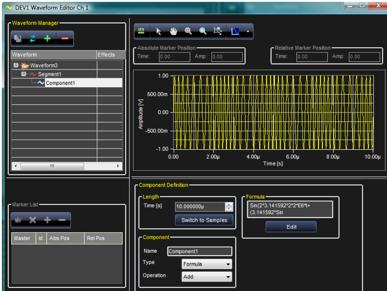
Figure 3-12. A phase modulation waveform. The actual formula used here is \text{Sin}(2*3.141592*2*2*E6*t+(3.141592*\text{Sin}(2*3.141592*0.4*E6*t))) . Set the time to 10.000000 μ to view the graph as previously shown.
