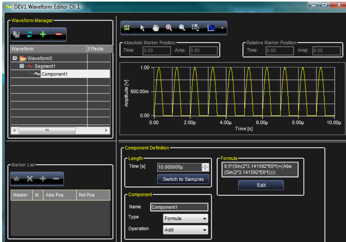
Figure 3-18. A half-wave rectified sine waveform. The actual formula used here is 0.5 * (\sin(2 * 3.141592 * E6 * t) + (\text{Abs}(\sin(2 * 3.141592 * E6 * t)))) . Set the time to 10.000000μ to view the graph as previously shown.
