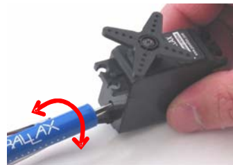
Gently turn screwdriver to adjust potentiometer
