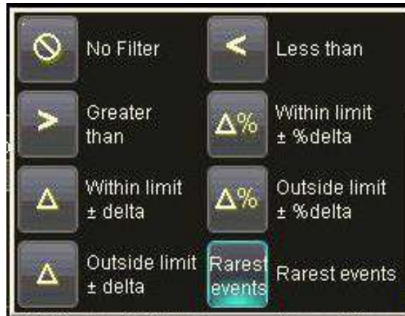
Figure 5: Triggering on signal conditions such as runts, pulse widths, frequency, rise/fall time, signal dropout etc. can be numerically filtered by a variety of user choices
