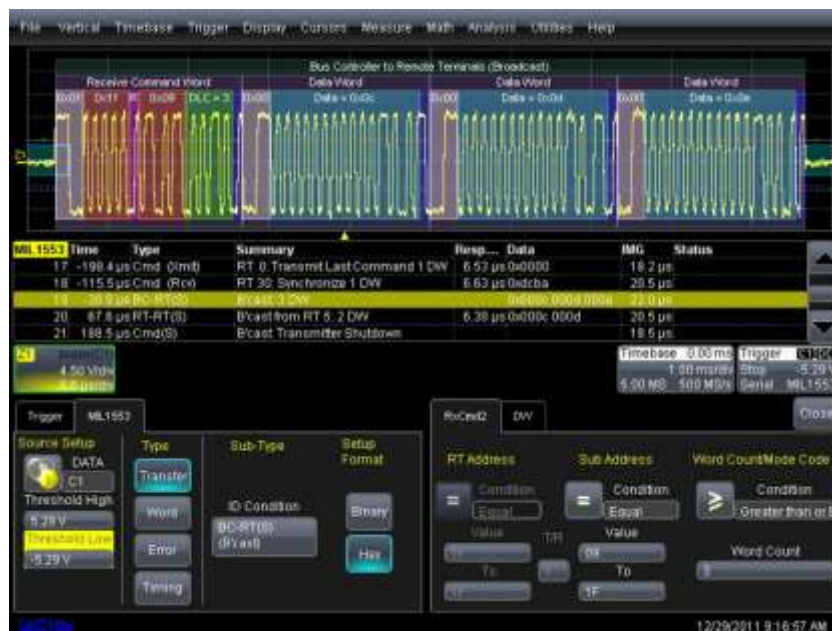
Figure 7: An example showing setup of triggering on a certain range of address values. The scope triggers and decodes the signal when an interesting address occurs.
