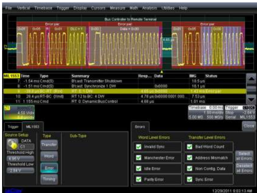
Figure 8: Protocol Aware Triggering and Bus Decode. In this case the scope is triggering on Error conditions
