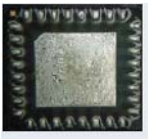
Figure 9 • X-ray Image Solder Voids
