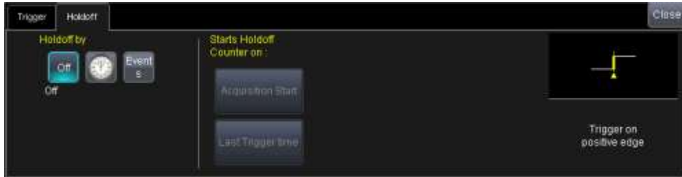
Figure 8: The Holdoff tab for setting trigger holdoff by time or events
