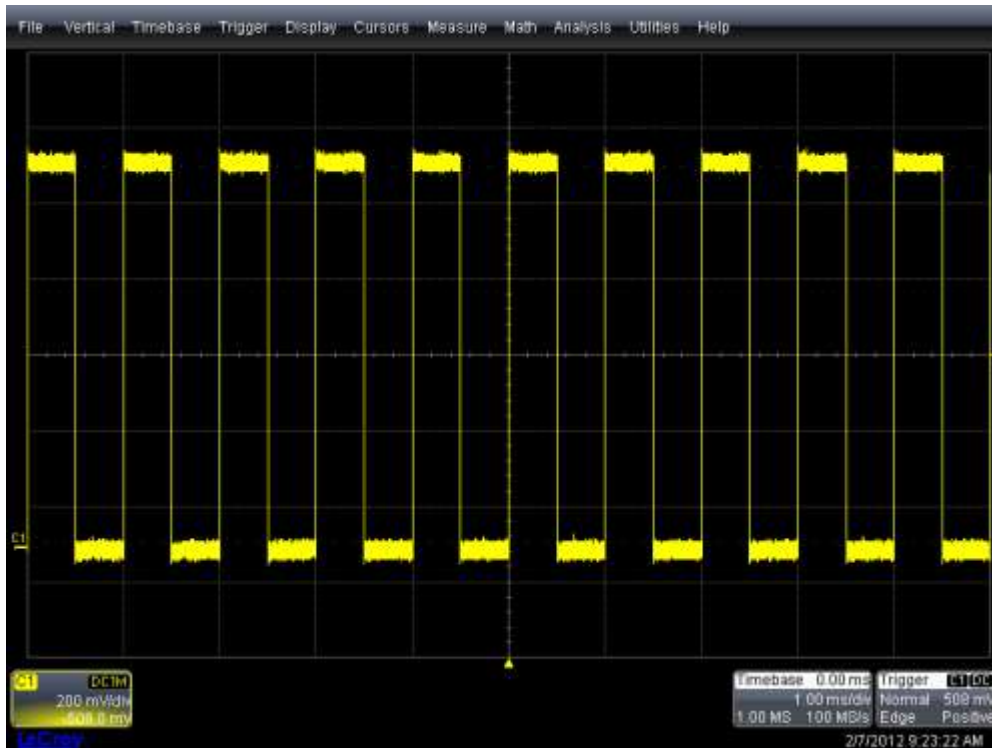
Figure 1: The initial setup of the oscilloscope showing the 1 kHz cal signal in channel 1
