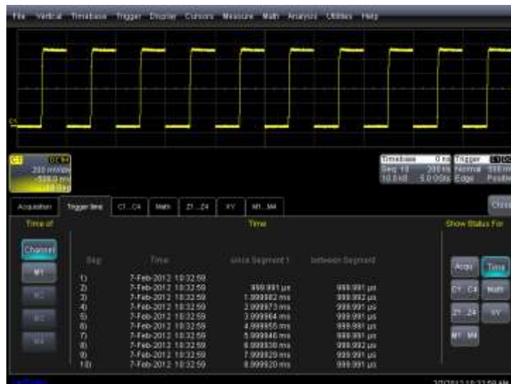
Figure 9: Using Sequence to time stamp each trigger
