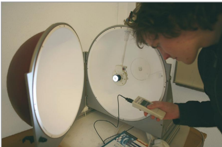
Figure 1: Measuring efficiency of a lens takes place in an integrating sphere.
