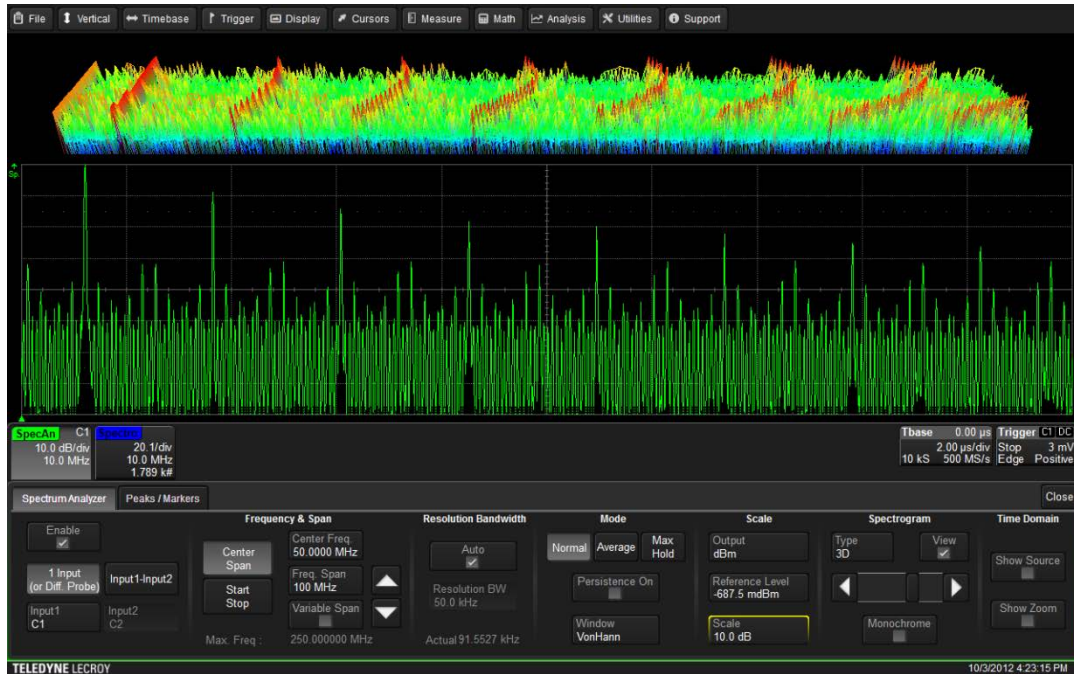
Figure 8: The 3D rendering of the spectrogram using color graded persistence
