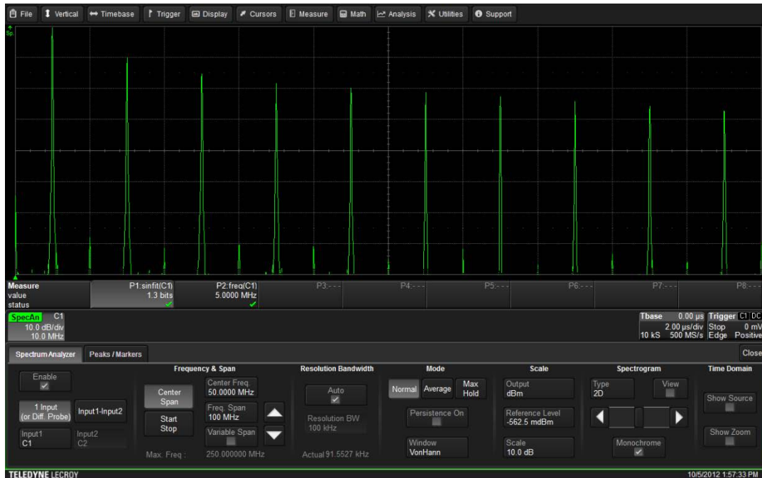
Figure 4: An example of a signal with greater than 12 bit resolution. An 8 bit scope would have a noise floor around 50 db below full scale obscuring the harmonics
