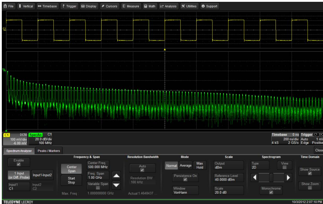
Figure 1: The Spectrum Analyzer dialog box showing the principal controls of the Spectrum Analyzer
