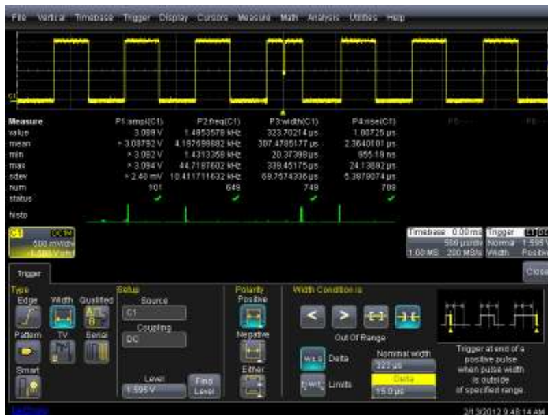
Figure 6: The second of two pulse anomalies revealed by the exclusion trigger setup
