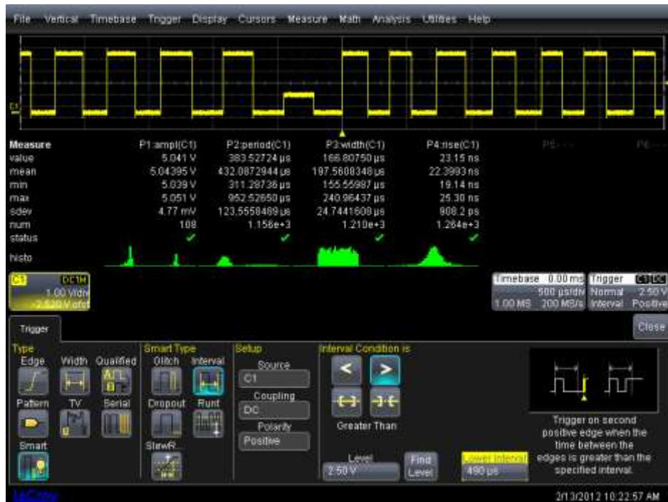
Figure 12: Using Interval SmartTrigger to capture the runt pulse
