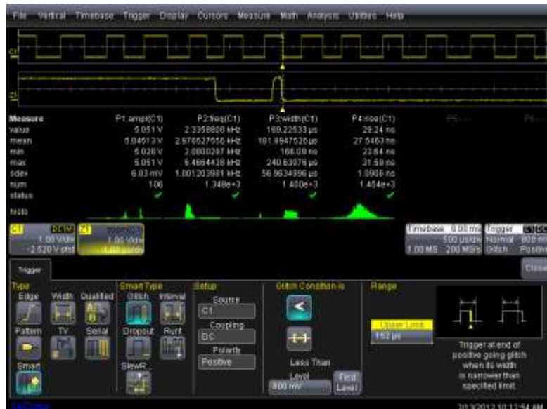
Figure 10: Using Glitch trigger to capture a 160 ns glitch
