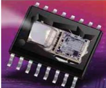
Figure 4. Example of using the MEMS sensing elements and the companion CMOS
