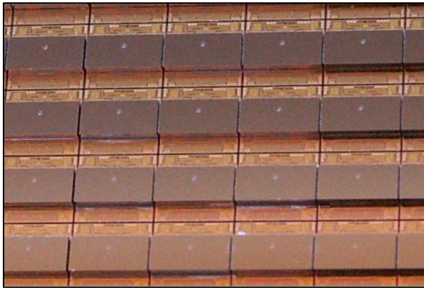
Figure 11. InvenSense's dual-axis gyro after dicing and pad
