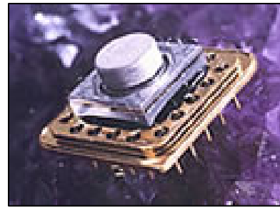
Figure 1. First generation electromagnetic MEMS vibrating ring yaw sensor by Silicon Sensing System
