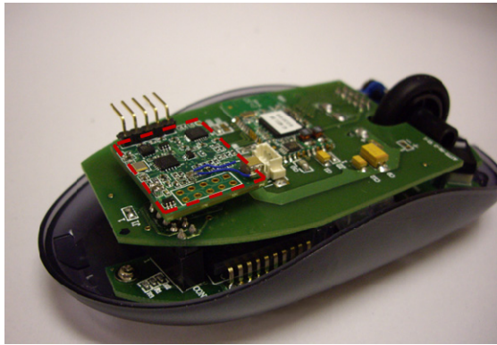
Figure 9. The InvenSense 9-axis reference board (outlined in red) has been retrofitted into a standard RF 2-D mouse, adding air-mouse functionality to the device.
